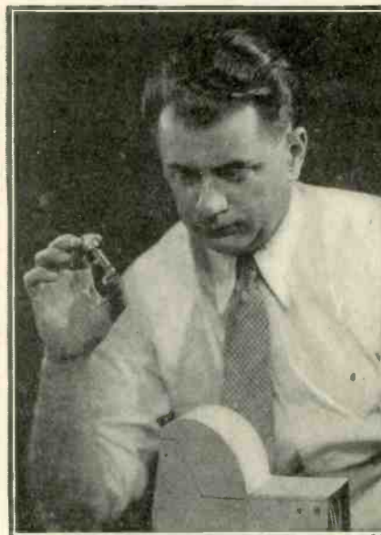
Small model of 30-line television receiver, employing the Scophony rotating-echelon principle. Actual size of television unit is easily visualised from this picture. The picture shows also the size of the moving part used in this type of receiver, which is held between the fingers of Mr. G. Wikkenhauser of the Scophony laboratory. This model, used with a mercury lamp, is capable of giving a satisfactory projected picture 3½ in. by 8½ in. and the moving part can be driven and synchronised by the output of a small valve.
