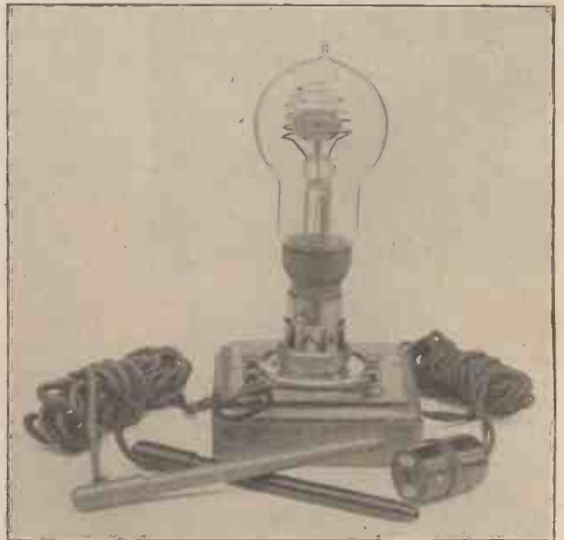
Not only is the neon lamp an essential part of television equipment but it can be made up into a form of tester with great ease.
