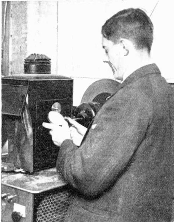
A tachometer is a very useful device for determining motor speed, but care must be exercised to impose no extra load on the driving mechanism.
