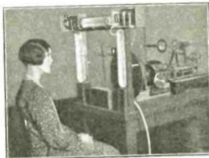
Fig. 4. A view of the television transmitting apparatus used by the American Telephone and Telegraph Company. Light from the arc lamp visible on the extreme right is condensed on the disc, which is driven by a high frequency synchronous motor. The disc carries a spiral of pin-hole apertures, each of which in turn projects a moving spot of light on the subject, as described by our Technical Editor in our last two issues. Light reflected from the subject is collected by the three large photo-electric cells.
