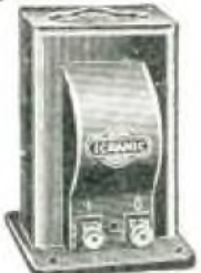
Igranic L.F. Choke, Type "G." The best low frequency choke made. Exceptionally high maximum inductance of 370 henries. By connecting the two sets of terminals in parallel an inductance of 80 henries is obtained. A really massive job. Price 27/-
