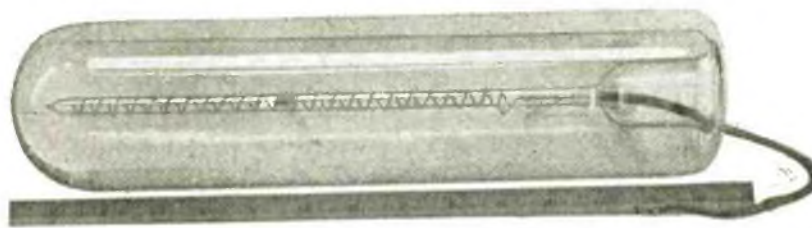
Fig. 3. One of the extra large photo-electric cells developed by the American Telephone and Telegraph Company. This cell presents 40 square inches of light-sensitive surface to receive light reflected from a subject being televised.
