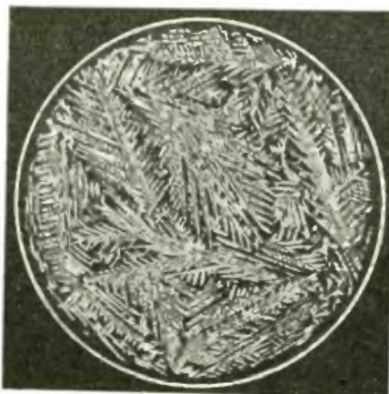
Fig. 1. Greatly magnified view of the normal edge of slab-selenium which has been cast in a shallow mould in a molten condition.
