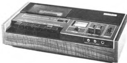
Also from Sony, the TC 127 cassette record/playback deck costing £69 15s is said to be the ideal companion to a hi-fi stereo system. Frequency response is given as 30 to 12,000 Hz and wow and flutter 0.2%.
