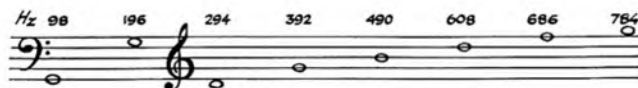
Fig. 2. The first note, G, is the fundamental. Those following represent an associated harmonic series
