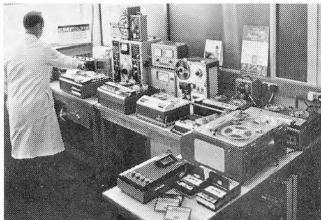
A small corner of the test area at the Emitape works, Hayes. Here engineers use the new Afonic tape on a wide range of ordinary domestic tape recorders under very much more severe conditions than would ever be encountered in the home. Application testing, as it is called, extends to cassettes and cassette machines
