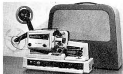
As an example of a magnetic stripe projector, the French Heurtier P6.24 S shown with combined carrying case/loudspeaker
