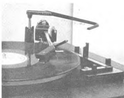
The BSR UA 70 Transcription Turntable fitted with type C1 ceramic cartridge
