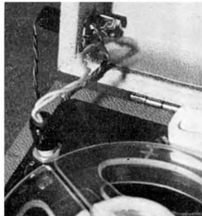
Above, shows earphone plug, reduced in size, with white lead going under covering material in lid. The miniature socket with jack plug inserted brings supply from auxiliary batteries. The lead from socket is inserted through filed-off corner of the deck
