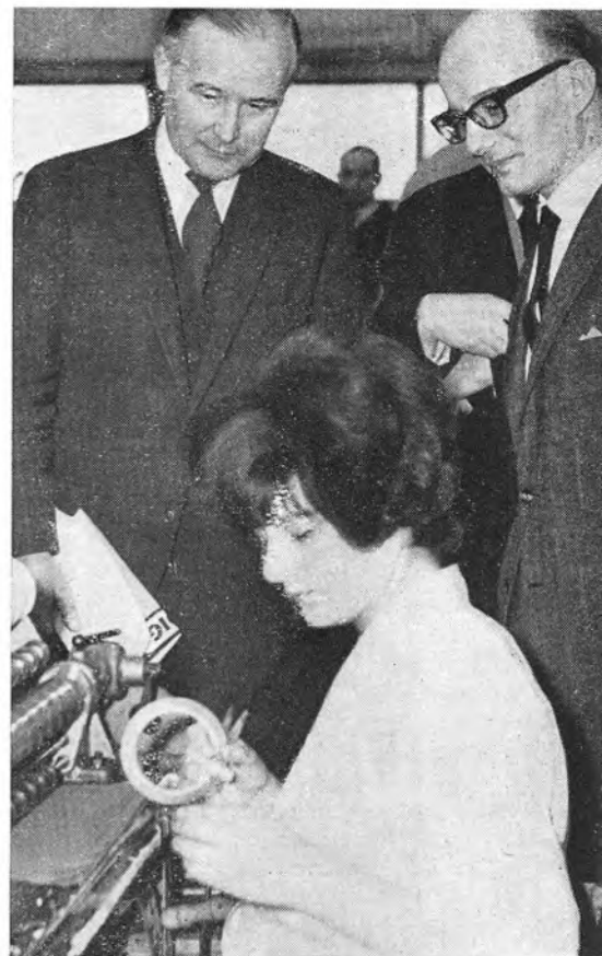
Mr. Paul Spring (right) Technical Director of Grundig (Great Britain) Ltd. and Douglas Brown, Editor of "TAPE Recording Magazine" watch coil winding for mains transformers. Ten coils can be wound in one foot-controlled operation
