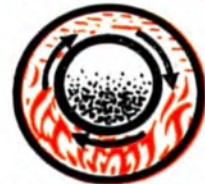
Section of the furnace, showing the magnetic oxide particles in the inner cylinder.
