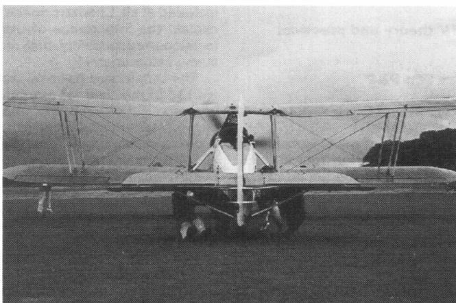
Holding down the tail of the display example Fairey Swordfish during an engine run-up at Old Warden. Godfrey Manning.
