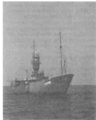
Fig. 4: Smith's Knoll Automatic light vessel. The automatic weather station is at the central mast-top above the light, The ship is painted red, masts and all!
