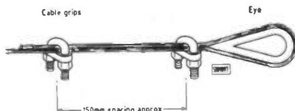
Fig. 3: Using an "eye" and cable grips to terminate a guy wire.
