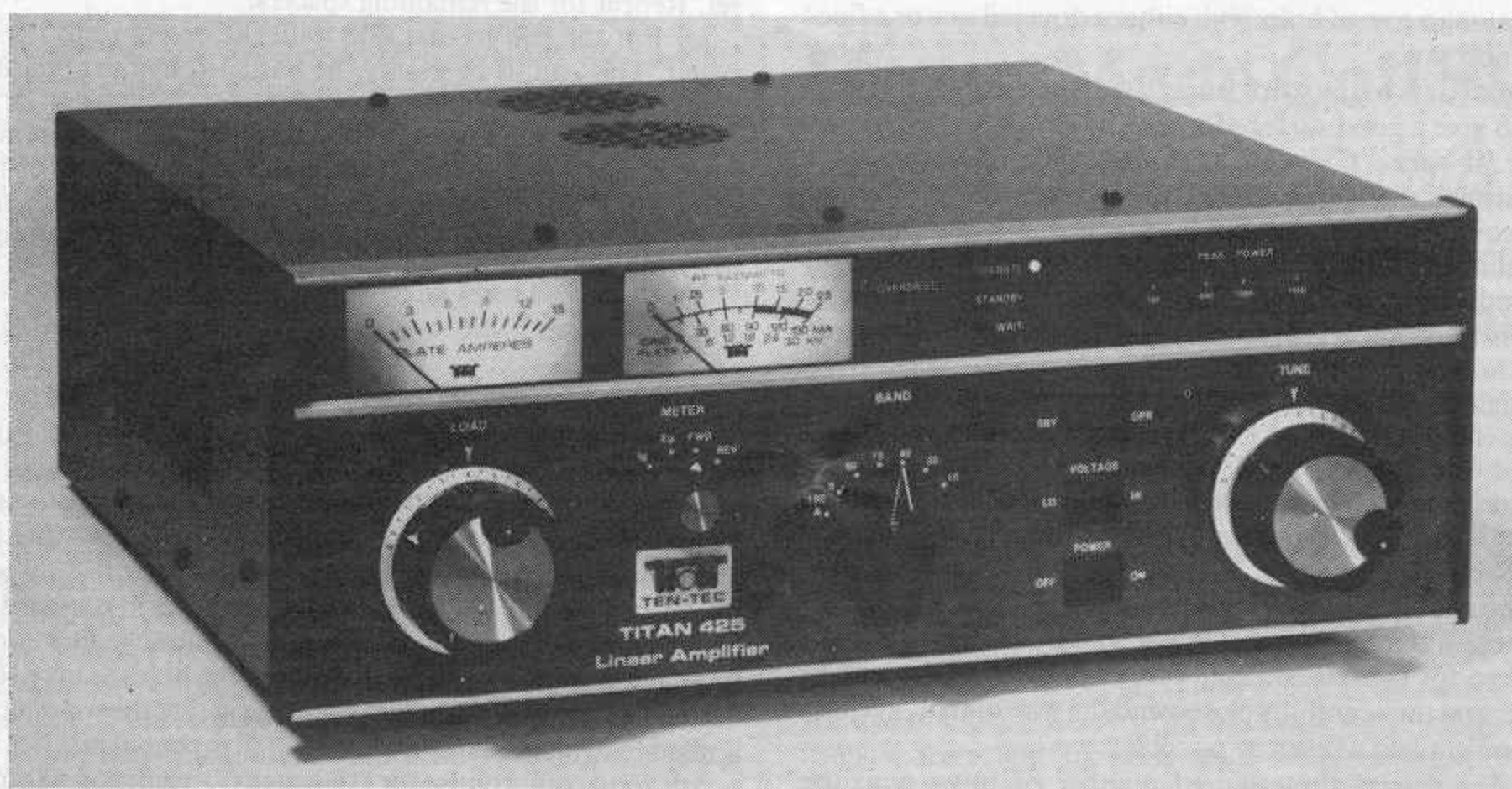
General view of the Titan linear amplifier. The export model (described) has an extra band switch position for 10 metres.
