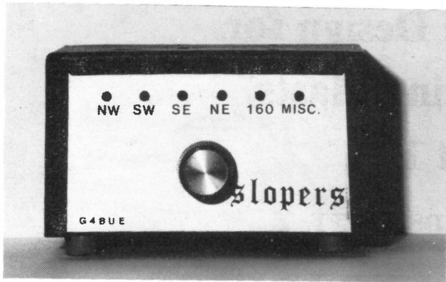
Photo D: The Control Box used for the relay box containing five relays and switching six antennas. Leds have been used to indicate which antenna has been selected.
