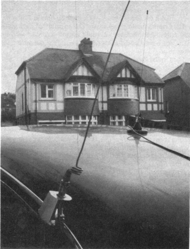
A view of the gutter-mounted 7/8-wave and mag-mounted 1/4-wave aeri-als.
