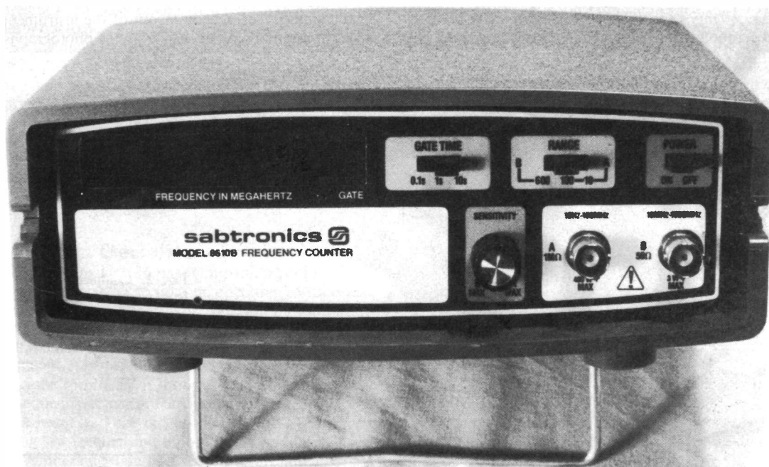
Fig. 1. The completed counter showing the clean, functional layout of the controls. The tiny hole just discernible beneath the letter E in 'Model' was drilled to gain access to the trimmer for adjusting the crystal oscillator frequency to exactly 10 MHz.
