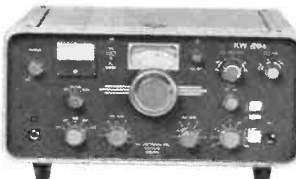
KW 204 KW 204 Transmitter. Well known for really good audio quality (SSB) and a favourite with CW enthusiasts. 10-160 metres. Reliable PA Tubes (2 x 6146).
