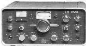
KW 2000E and Power Supply KW 2000E Transceiver covers all HF Bands 10-160 metres (10 metres in 4 Bands), 500 kHz VFO. SSB/CW. Outstanding TX audio quality. Excellent receiver signal-noise figures. Includes VOX, break-in CW, 100 kHz and WWV calibrator. Reliable 6146's in P.A.
