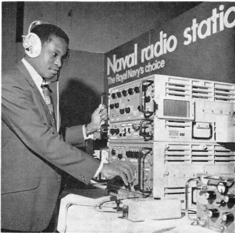
The Redifon main radio ship station Type 643 has been adopted for fast patrol vessels of the Kenya Navy, of which Maj. J. Kibwana is chief communications officer. The transmitter is all-solid-state, CW and phone, and runs 100w., with a companion receiver Type CJP. The Royal Navy is also taking these installations, for which a 400-watt broadband linear is available.
