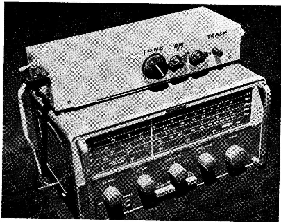
The PLL unit, as used by G3HMO and discussed in the article, is in a chassis which sits on the EC-10 main Rx. Controls are explained in the text, except that the small central unmarked switch selects a range of capacitors for varying the bandwidth of the LFF.
