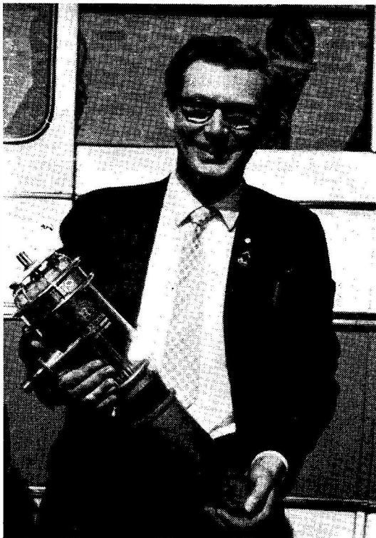
Just one of the ordinary modulator valves as used by the BBC on some of their transmitters. This was an "out of hours" specimen presented to the chairman of Northern Heights as a memento of the Club's recent visit to the BBC's Skelton Pastures Tx station in Cumberland. This is the sort of bottle that needs about 100 amps. on the heater and 5000v. on the plate!
