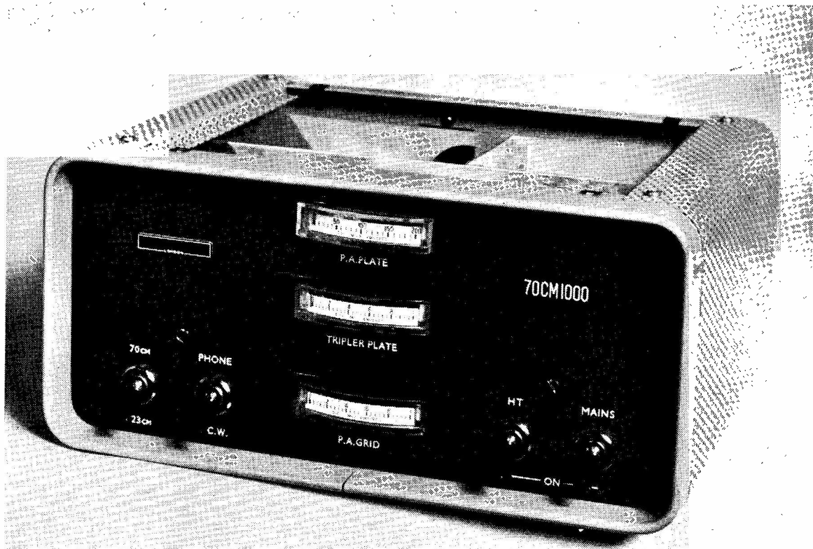
The Green & Davis 70CM100 is a tripler-amplifier for the 430 mc band, rated at up to 90w. input, depending upon what PA valve is fitted (to customer requirement). Both tripler and amplifier stages are blown, and all 70-cm. circuits are formed by parallel lines, screened for better efficiency and minimal radiation. Both stages are metered, a heavy-duty coax relay is fitted for aerial change-over, and all metal-work relevant to the output frequency is heavily silver-plated. Construction is on a copper chassis. The 70CM100 is intended to be driven from any suitable two-metre transmitter.
