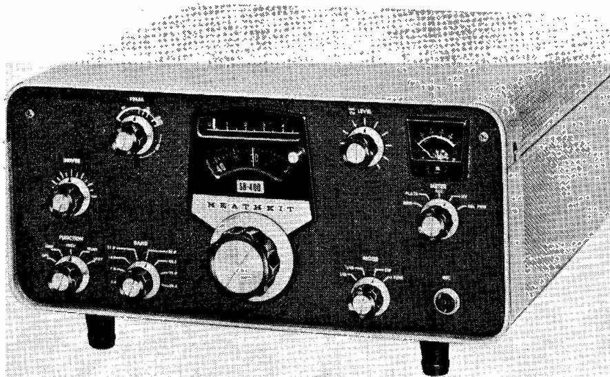
The new Heathkit Sideband Transmitter, Model SB-400, is a very interesting piece of equipment, now making its debut. It is a five-band Tx, covering 3.5-30 mc in the amateur ranges, and giving 100w. RF output over 15-80m. and 80w. on 10m., into a 50-ohm load. The SSB rating is 180w. p.e.p. and 170w. on CW, adapted for break-in, using grid-block keying. Sidebands are selectable, and the specification shows a very high order of frequency stability. The PA is a pair of 6146's, and the PSU, using silicon diodes, is self-contained.
