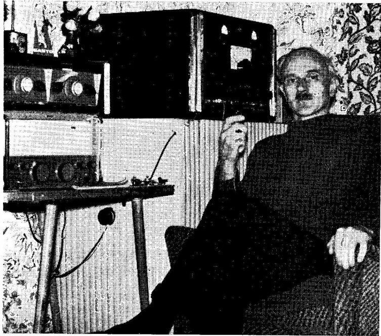
Now of 34 Birch Avenue, Romley, Cheshire, G4HU was first licensed pre-war under the AA call 2DDM. After a varied experience, on the air and off it, he is now settled on 14 mc for CW and 3.5 mc for phone, operating after midnight because the local TV receiver time-base radiation blots out his Rx—TVI in reverse. In fact! The Tx is a PR-120V and the receiver an Eddystone 840C with a Codar PR-30X preselector and a Q-multiplier. For the HF bands the aerial is Mosley trapped dipole, with "a bit of wire" for 80m. G4HU's other hobby is fencing and, taking part in tournaments about the country, he travels /M.
