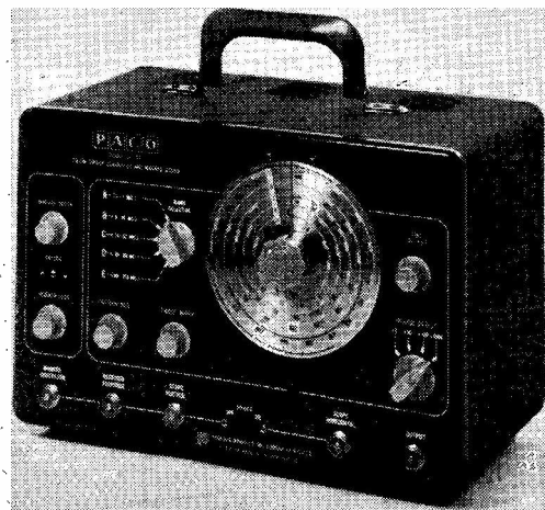
The PACO G.32 Sweep Generator is an FM Sig. Gen. with a basic frequency range of 3-213 mc in 5 bands overlapped, and the sweep width is adjustable over 0-30 mc at the VHF end. The application of the instrument (which is available in kit form) is in the alignment of wide-band amplifiers, and a marker-adder facility is provided to avoid misleading results.
