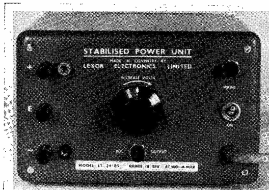
The Lexor stabilised power unit for low VA supplies has a continuously variable output voltage control—in the ranges 5.5-14v. or 18-28v., depending on the model selected—and is capable of delivering output currents up to ½-amp. at any voltage setting within the chosen voltage range, with regulation better than 0.15% for a 10% mains voltage change, and within zero to full load. The finished mounting is a steel instrument cabinet 8ins. wide, in grey stove enamel.
