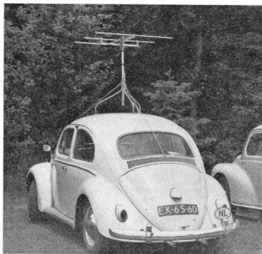
PA0CY/M (from The Hague) was at the Hasselt Fox Hunt; he has a 3-element array for two metres, mounted on a support held to the roof of his car by rubber suction cups. The Fox Hunt involved searching for a hidden two-metre transmitter.
