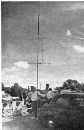
When G5PP (Coventry) wants to work /P with his mobile installation he can put up, from the car, a two-metre beam and a loaded whip for 160m. The whole assembly knocks down into handy sizes. A G3GMN print
