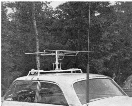
Seen at Hasselt, Belgium, on June 24, for the International Fox Hunt. DJ5KQ/M (from Juelich) has an all-band whip of conventional design plus a 4-element Yagi for two metres, which can be rotated from the driving position!
