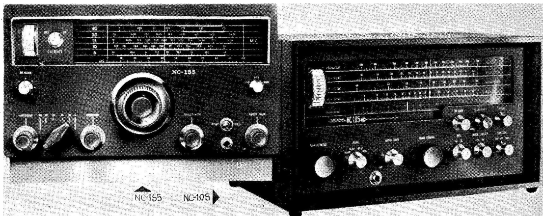
On the left, the new (American) National NC-155, an amateur-band double conversion superhet with full spreading over the bands 80-6 metres (3.5 to 50 mc); variable IF selectivity from 0.6-5.0 kc; a sensitivity claimed to be better than 1 μV for a 10 dB signal-noise ratio; and what is described as "planetary 60:1 tuning." For SSB reception, there is a separate product detector, sideband AGC, and a BFO calibrated for USB/LSB. Other features are band-edge calibration, automatic noise limiter and an edge-reading S-meter which follows on all reception modes. The receiver on the right is the National NC-105, a general-coverage design in the same category, having a frequency range of 550 kc to 30 mc in four bands. It also has a Q-multiplier, a product detector and a series gate type noise limiter. Calibration charts are supplied for the amateur and broadcast short-wave bands.
