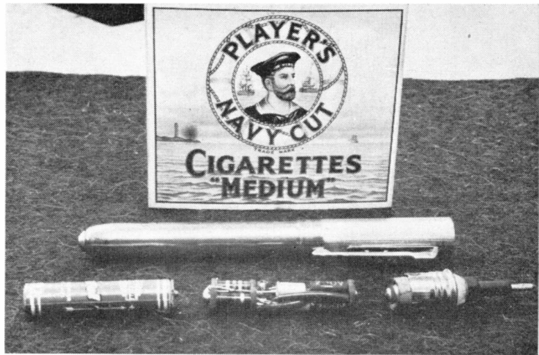
This view of the pen-torch tester in its component parts shows the assembly on the formers sketched with the circuit diagram. It should be noted that in this photograph the battery is shown wrong way round — it should be negative (case) end to resistor contact button.
