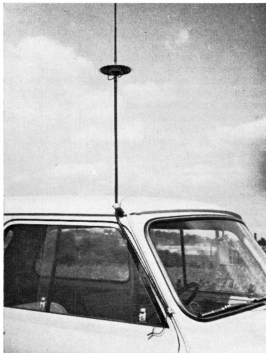
Showing the upper and lower bracket mountings for his Top Band aerial on G3BMN's car, an Austin Mini-7. The coil design is described in detail in the article.
