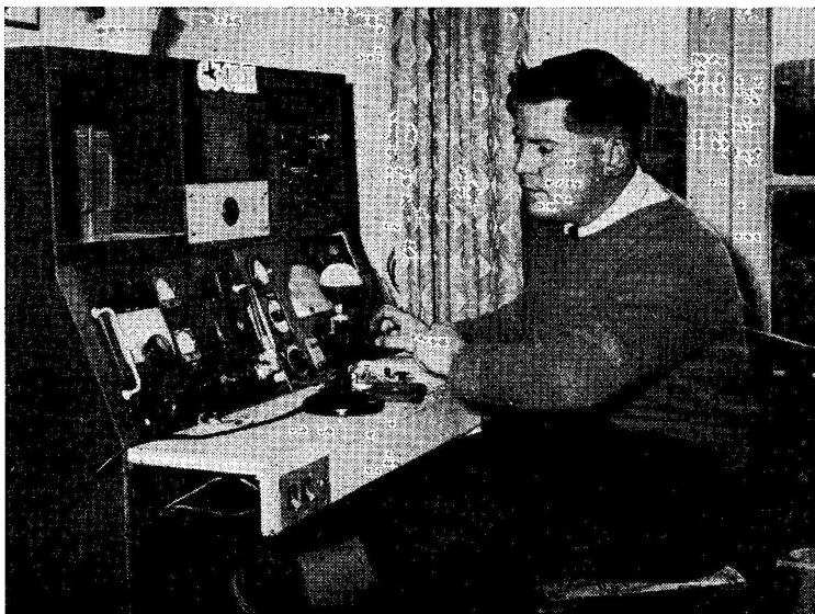
G3OMH is operated by D. Hayward at 6 Larkhill Road, Yeovil, Somerset, and with the exception of the Eddystone 358X receiver, all gear is home-built and based entirely on "Short Wave Magazine" published designs; the main transmitter runs 80w. to a pair of 807's and covers 10-80 metres, for which the aerials are a 67 ft. wire and 20-40m. dipoles. Full BK facilities are provided for CW working, and the whole station is contained in the cabinet seen in the photograph. G3OMH/M is also constructed to Magazine designs, the transmitter being an adaptation of the "Top Band Talking Box" (October, 1956) with an 8 ft. centre-loaded whip and modified Command receiver.
