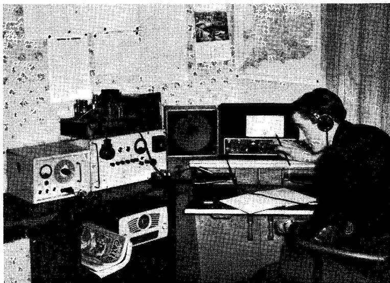
Neat layout at the SWL station of D. Hanson, 26 Tomlin Avenue, Mirehouse, Whitehaven, Cumberland, and entirely home-built except for the Eddystone S.640 main receiver. Chief interests are in the 14-21-28 mc bands, for which a pre-selector (extreme right) is available, the aerials being 67 ft., 132 ft. and a dipole for 10 metres. Other items of equipment include a multimeter, stabilised power supply unit, and an 8-watt amplifier.
