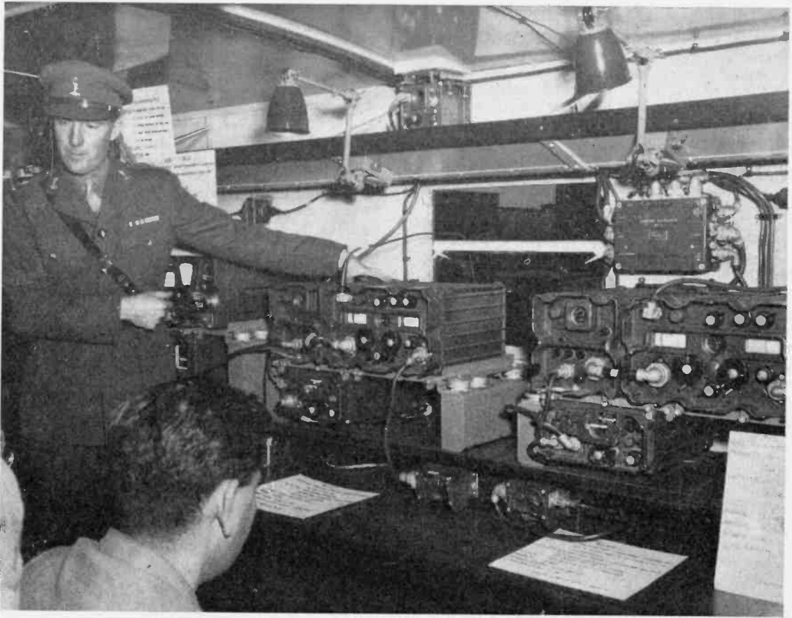
During a recent visit to the Plessey factory at Ilford, a number of Service representatives were given a demonstration of the new Plessey military-vehicle VHF communication equipment. This is designed to withstand hard usage and certain of the sets have already been adopted by the Army and the Royal Air Force.
