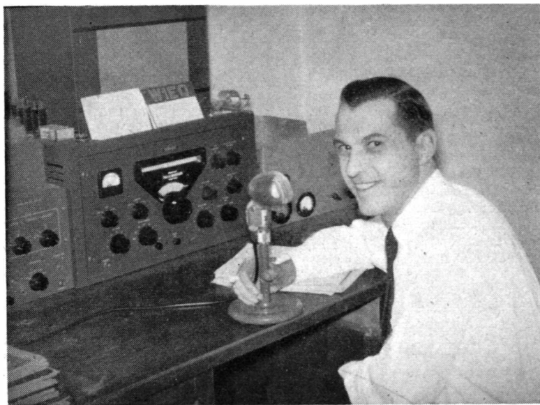
Station of DL4SV/W1EO, Munich, with a GG Linear RF amplifier consisting of a pair of 837's driven by a 20A sideband exciter. His receiver is a Collins 75A-1.
