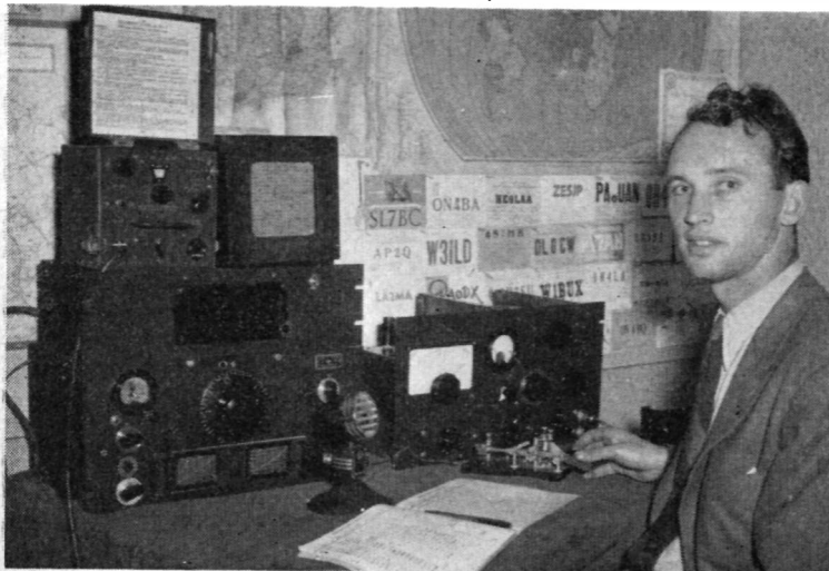
G3IFB, Kenton, Middlesex, was licensed in March, 1952, and now has 125 countries worked in 37 zones, gained mainly on Ten/Twenty, using CW. The transmitter runs 807's in the PA, at 150w. input and for phone the modulator is a pair of 807's in Class-B. The receiver is an HRO-5 and the aerial is cut to be 3-half-wave on the 14 mc band (102 ft.), fed at a low-impedance point through 80-ohm line.
