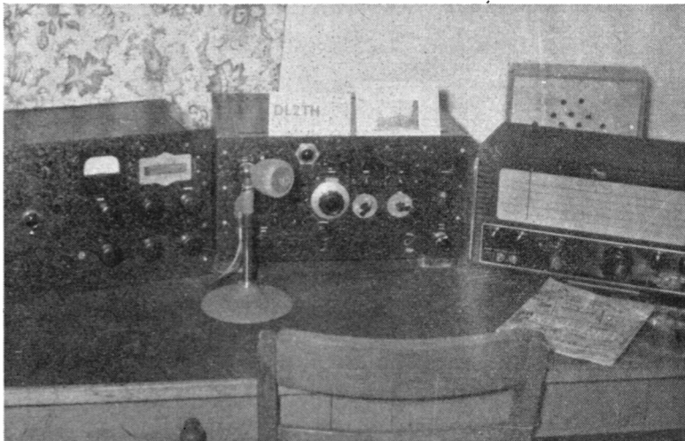
When in Germany, DL2TH/DL2YL ran a husband-and-wife station, and were on SSB. At centre is the home-built alidband exciter, giving about 30 watts peak output, driving the linear amplifier (left) using three 807's in parallel. The whole transmitter assembly is band-switched for 80-40-20-15-10 metres; over 900 SSB contacts were made with this rig, and the Eddystone S.750 receiver at right. DL2TH, who was at one time VS1BQ, is now under way again as G3HSR.
