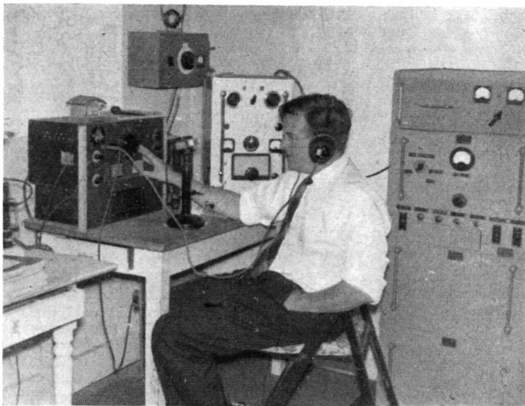
G3KQP of East Molesey has been licensed for two years and is regularly active. The transmitter in the centre-background is a Chinese copy of the LG-300, entirely home-constructed (by G3KQR) powered from and modulated by a modified T.1131, in the rack to the right. The receiver is an HRO, and on the wall is the all-band aerial tuning unit, which also includes a dummy load. The T.1131 relay system has been adapted for the change-over control.
