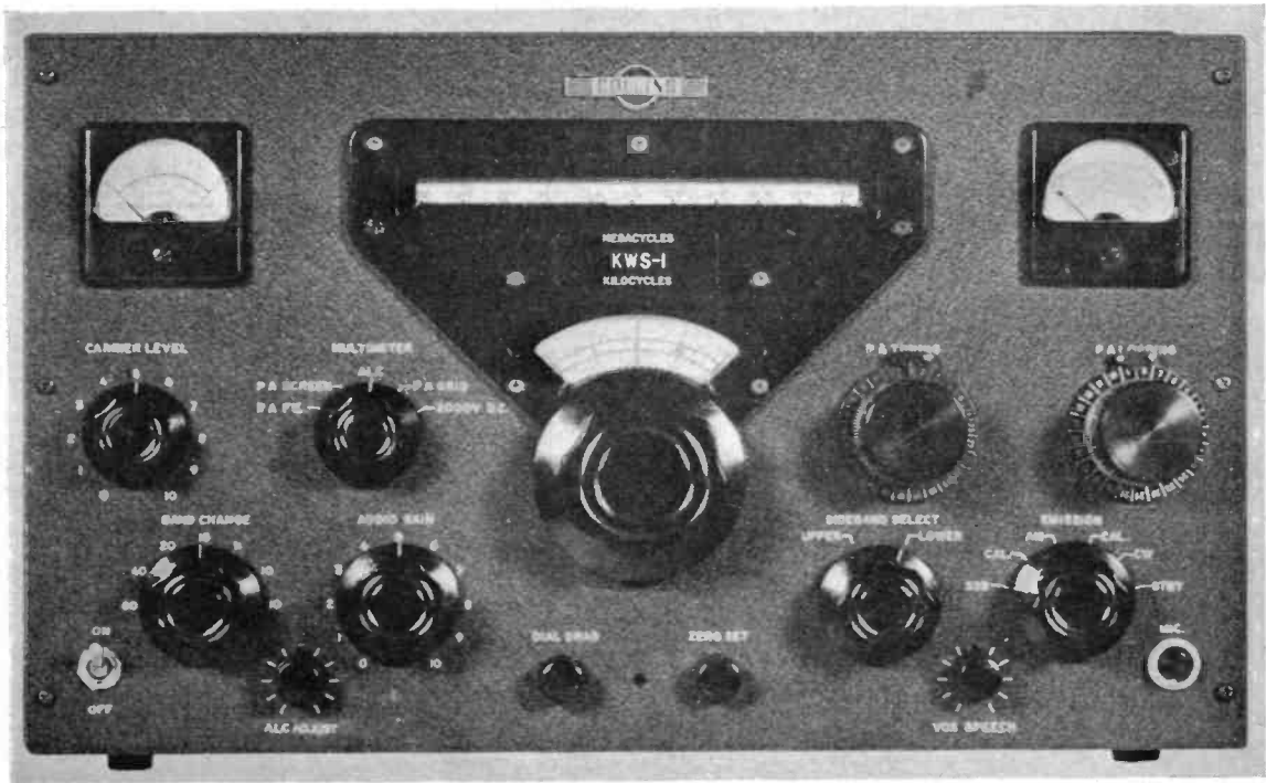
Front-panel arrangement of the KWS-1 AM/CW/SSB Transmitter, manufactured by the world-famous Collins Company of Cedar Rapids, Iowa. The KWS-1 is a table-top design rated at one kilowatt and though designed for the American amateur market, has already found a number of commercial applications.
