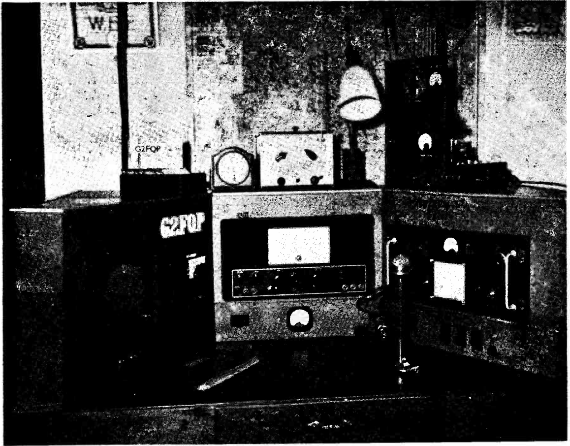
The console layout at G2FQP, Ramsey, Hunts., an active VHF station in a sought-after county. The 2-metre receiver is a crystal-controlled G2IQ converter into an S.640, shown here, and the transmitter runs 20 watts to an 832 on 144.72 mc.
