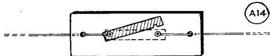
Fig. 3. Patch board or strip connector in series with the radials, for altering their length (see text).
