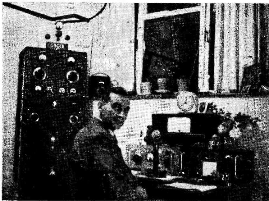
Station of G3GIR, Gorleston-on-Sea, Norfolk. Frequency control is by Heterodyne Crystal Oscillator-VFO, using a 6F6 through two 6V6's as buffer-doubler; the PA is a pair of PT15's driven to 150 watts by an 807, modulation being by cathode control of the PA with a pair of 807's. The receiver is an S.640 and main interest at G3GIR is 14 mc phone and CW operation.
