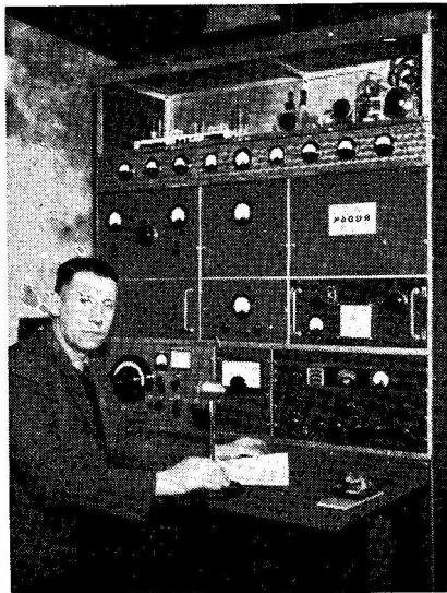
General view of the station of PAØDR, Middelstum, who has a rack of his own design carrying transmitting and receiving equipment for the Two, Ten and Eighty Metre bands.
