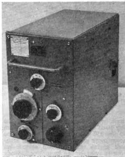
General view of the Type 145 Oscillator. Controls are : Bottom left, vernier shift ; middle left, main dial ; upper middle, tank trim ; upper right, wave-change. Lower right is the crystal holder.
