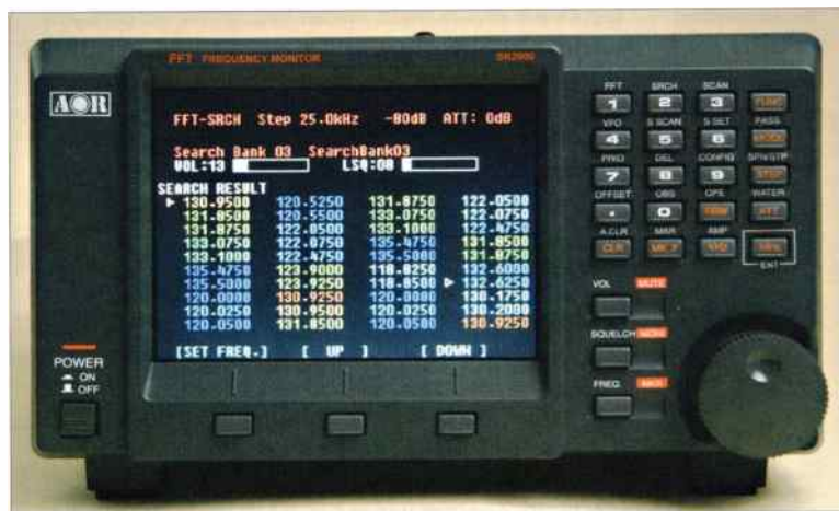
● Fig. 5: The FFT search lists its results in eight different colours to show the relative signal strength.
