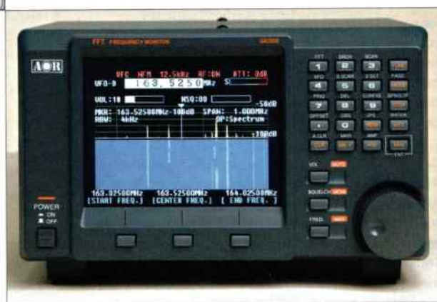
● Fig. 7: The waterfall display shows signals over time. Here we see activity in a busy PMR band.
