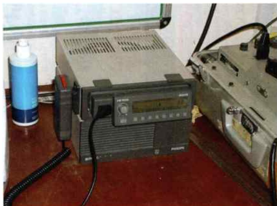
■ A Philips FM1000 v.h.f. set for the marine bands also to be found in the h.f. shack.
