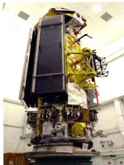
■ Fig. 10: NOAA-N satellite prior to enclosure - showing the solar panels folded.
