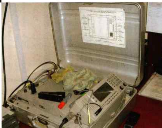
■ A closer look at the Marcom transceiver for chasing some interference.
