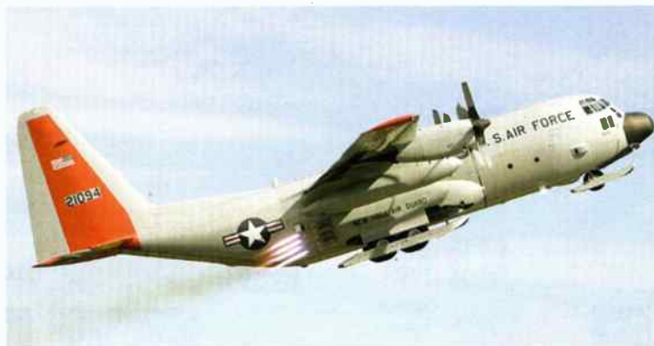
LC-130H Hercules (USAF Air National Guard) Operating from New York, this grey and orange coloured Hercules transports equipment and personnel to Antarctica - hence the skis! Expect to see one in the flying display and then one in the static park, which can be viewed up close. Rarely seen but always welcome at the Tattoo. Picture by Dariusz Jezewski 'FotoDJ'
