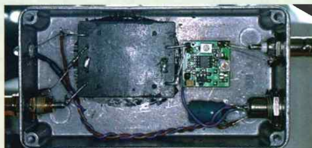
Fig. 4: The housed module and isolation transformer.
