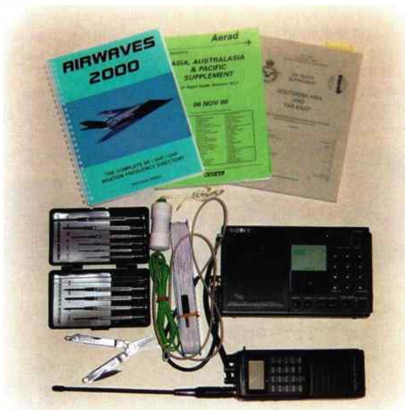
The components of my 'radio station' while in India - h.f. receiver, scanner, frequency guides, a small toolkit and a portable red-wire antenna.
