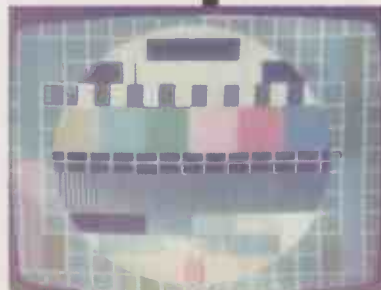
Fig. 4: This month's 'Down Memory Lane' item: the BBC Test Card 'G' (based on the PM5544, but with a modified grey-scale and central black bar), photographed in the Seventies.
