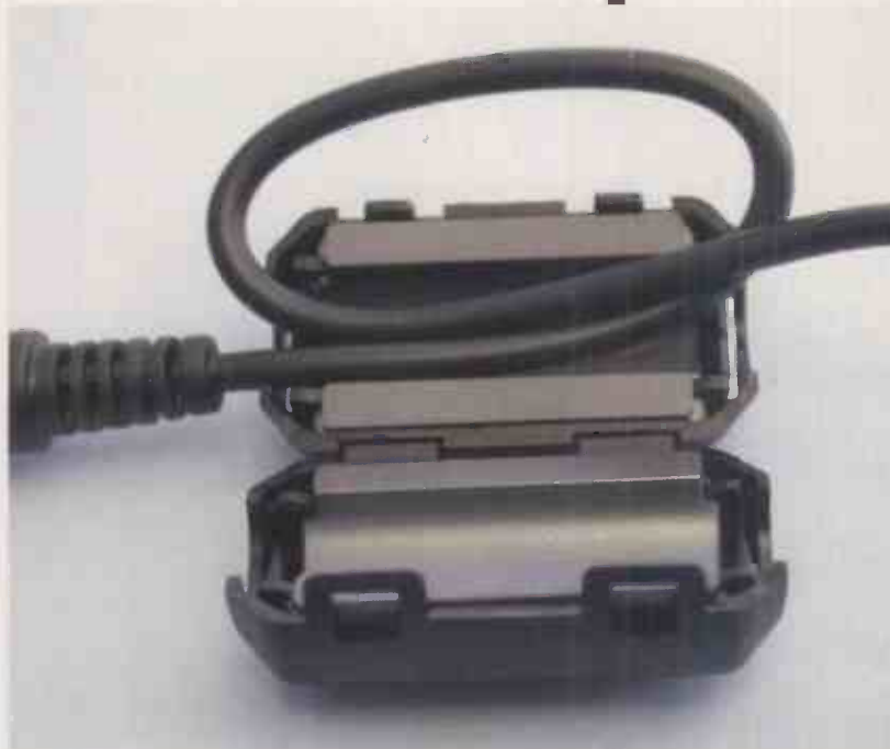
Inside a clip-on ferrite choke.
