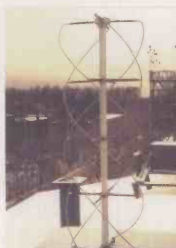
Fig. 4: QFH antenna used for the 137MHz band transmissions.
