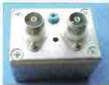
A fully-screened tunable Band I notch filter, a vital tool to remove interfering signals.
