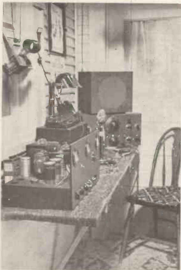
The rig at W5RG, Dallas, Texas, who runs only 18 watts to an 807 final, on which he has worked nearly 70 countries.
