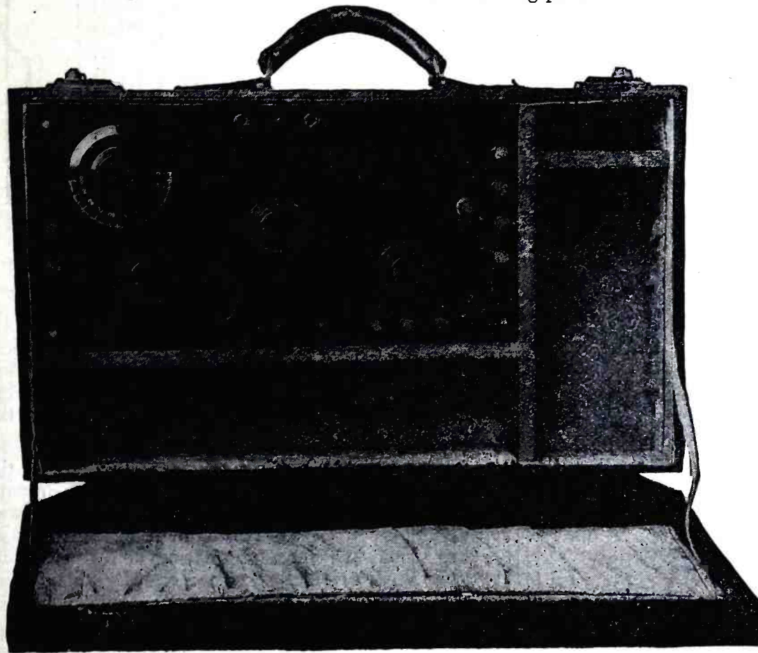
The set can be installed in a regular week-end case with wooden partitions as shown. The loop may be fixed in the cover of the case.
