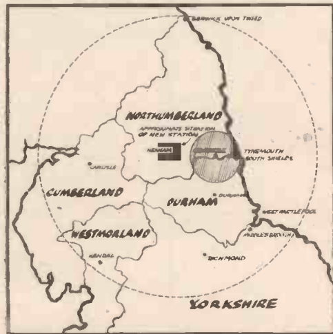
★ The shaded section shows the area at present served by the Newcastle transmitter. The wide circle indicates the immense range of the new Stagshaw transmitter.
