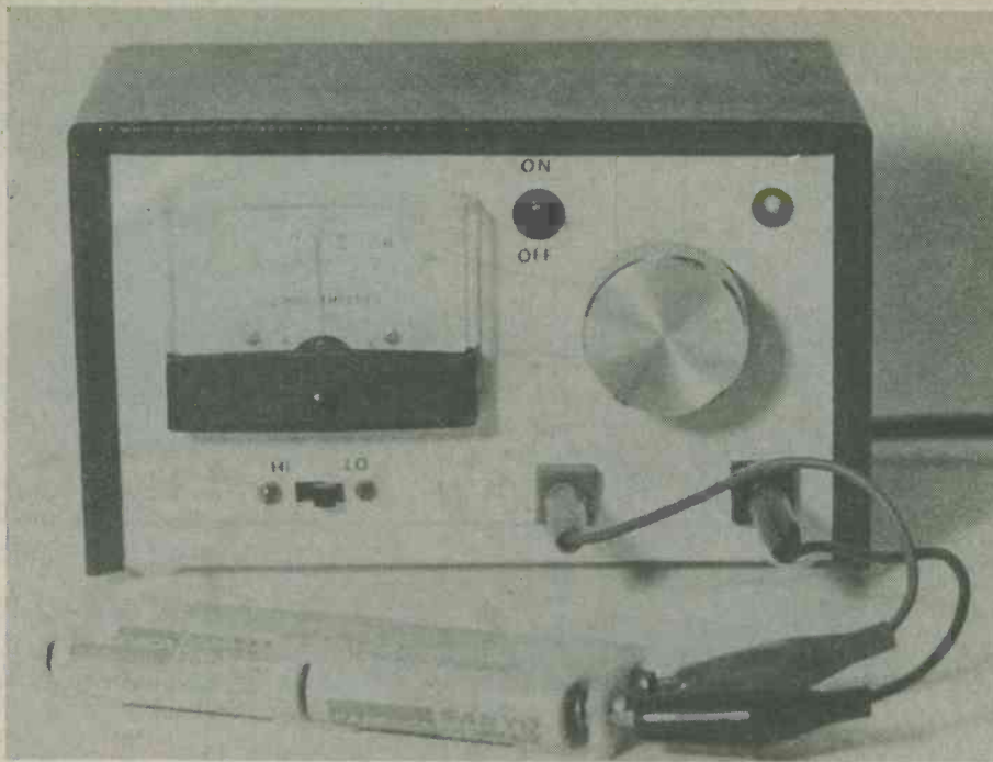
The charger in use. Here it is charging four HP7 size Ni-Cad cells
