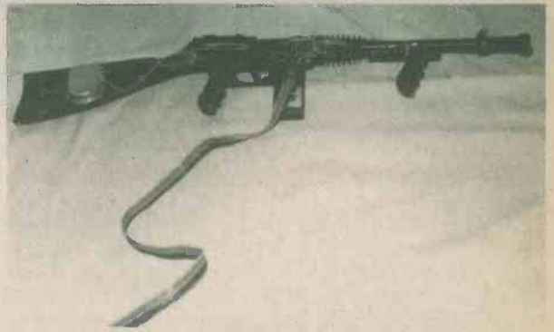
The miniature speaker is fitted in the butt of the gun. The gun flash i.e.d. LED1, is mounted on the top of the gun housing, slightly forward of the butt, so that it can be seen by the marksman. The 12-core lead has an anchorage at the "magazine", and in the area above this is fitted the electronics, apart from the trigger switch and the photo-electric cell
