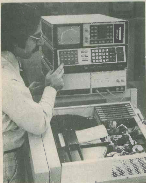
The new Hewlett-Packard Model 5420A Digital Analyzer in operation. Here it is determining the control system characteristics of a disc memory
