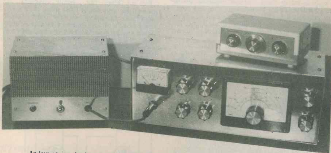
An impressive short wave receiving installation. Here are the 3 Band Short wave Superhet, the Eliminator-Speaker Unit which was described last month and this, and the 3 Band Preselector
