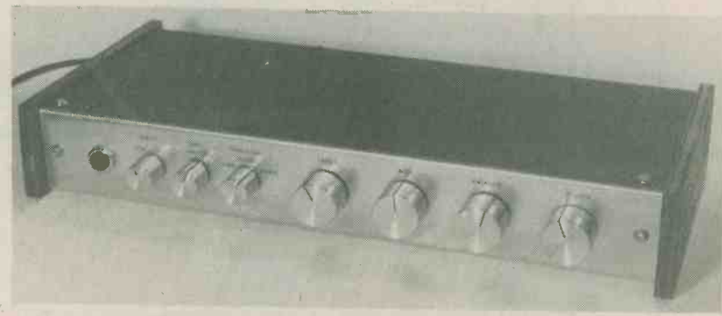
The stereo amplifier is housed in a shallow commercially available cabinet, thereby combining ease of construction with optimum presentation
