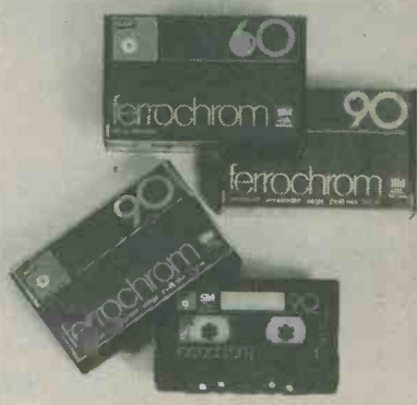
BASF cassettes incorporating Ferrochrom tape. This has a layer of ferric oxide on the tape base, with a carefully controlled layer of chromium dioxide above.
