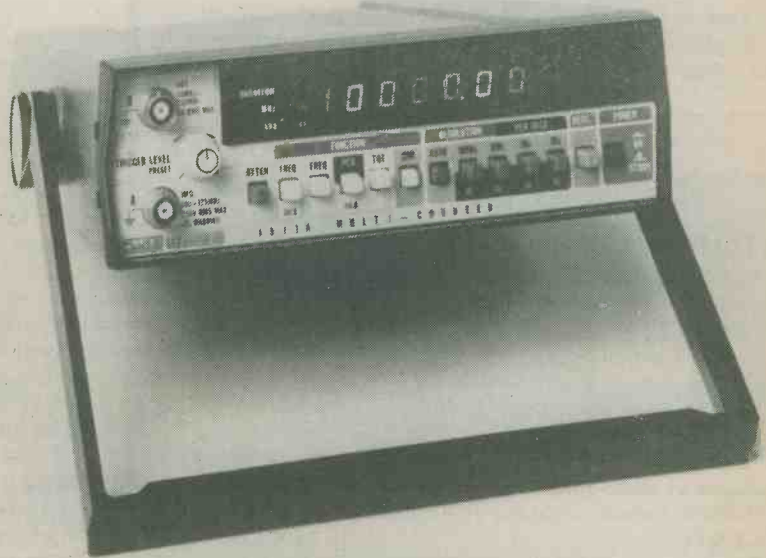
The Fluke Model 1911A frequency counter. This has a range of 5Hz to 250MHz, and offers a 50\Omega input impedance from 50MHz to 250MHz. Input sensitivity over most of the range is 15mV
