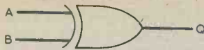
Fig. 2. Circuit symbol for a 2-input exclusive-OR gate. This truth table is given in Table 1
