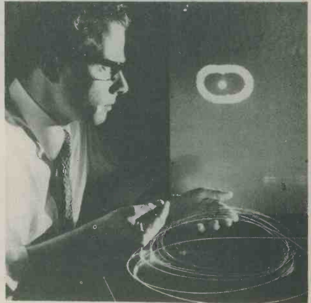
A Bell Laboratory scientist views the effects of light transmitted through the new glass fibre. Its structure makes it possible to take full advantage of the extremely low-loss light carrying capabilities of ultra-pure glasses
