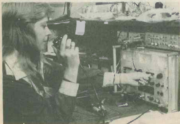
Test technician aligns the CQP 800 and checks transmit watts and receiver sensitivity across the complete frequency band.
