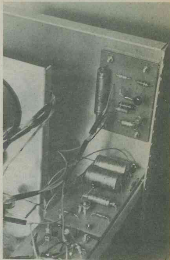
The flyback blanking amplifier board is fitted to the rear panel of the case, above the 12 volt supply board
