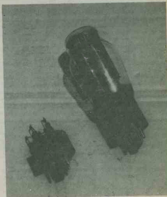
A valve rectifier and the plug-in rectifier unit which replaces it
